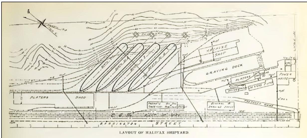
**The planned layout of the Halifax Shipyard circa 1919 following the 1917 Halifax Explosion**
