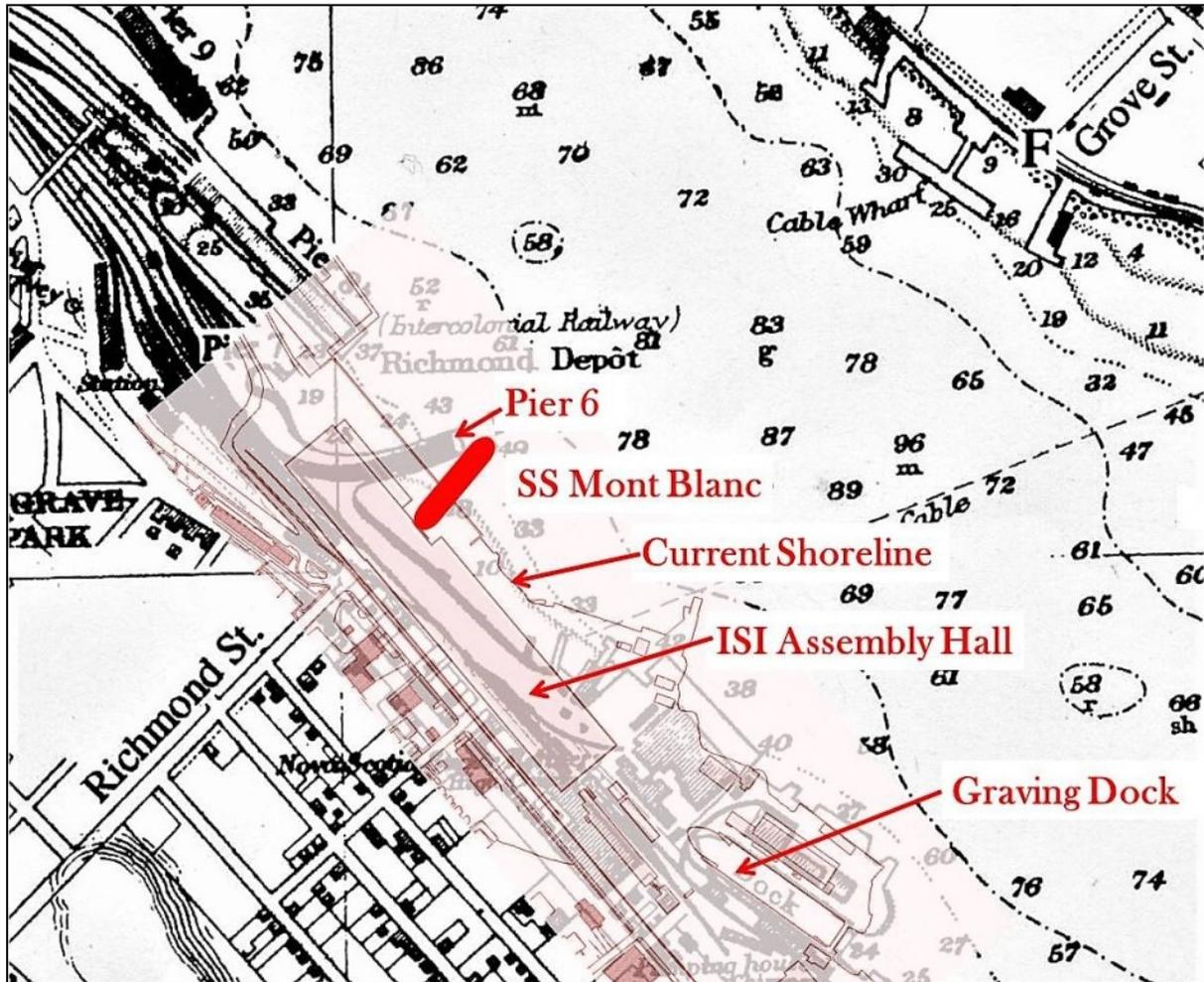
British Admiralty Halifax Chart 1416 (in black) showing the locations of Pier 6, SS Mont Blanc and SS Imo, overlaid with a scale site plan of the current Halifax Shipyard (in red), illustrating their relative positions
