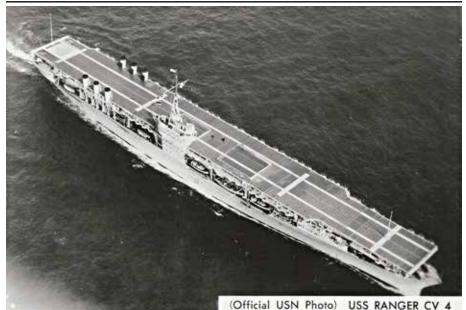
This 1934 photo shows many of *Ranger*'s defining features and many that would be changed over time. For example, note the two 5"/25 guns on the forecastle. Similarly, two of the guns are on the stern. This original arrangement was intended to give greater fore or aft concentration of the 5"/25 battery. However, soon the guns on the forecastle and stern would be moved to the four corners of the flight deck – where the guns would remain until fully removed by July 1944. (Flickr)
