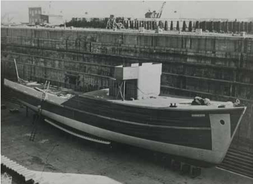
RCN Bay-class minesweeper HMCS Gaspé under construction at Davie Shipbuilding, 1951. The photograph shows the composite wood and aluminum hull, intended to help reduce the ship's magnetic signature. (Credit: CWM 19650068-009_58, George Metcalf Archival Collection, Canadian War Museum)
